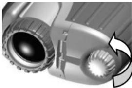
Open the door to install batteries
